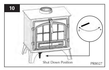
• Lowest possible heat out put for burning wood. This position does not keep the glass clean, Diagram 10
